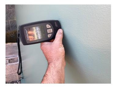
60K West Tank - Dry Film Thickness Measurement
