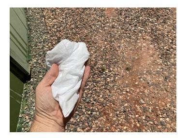
Clean cloth used to verify removal of chalking and contaminates. Surface cleanliness acceptable.
